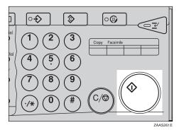
The machine calls the destination. While it is dialing, the number or name which is programmed as the RTI or CSI in the machine of the other party is shown on the display. When connected, the machine starts scanning the original.
